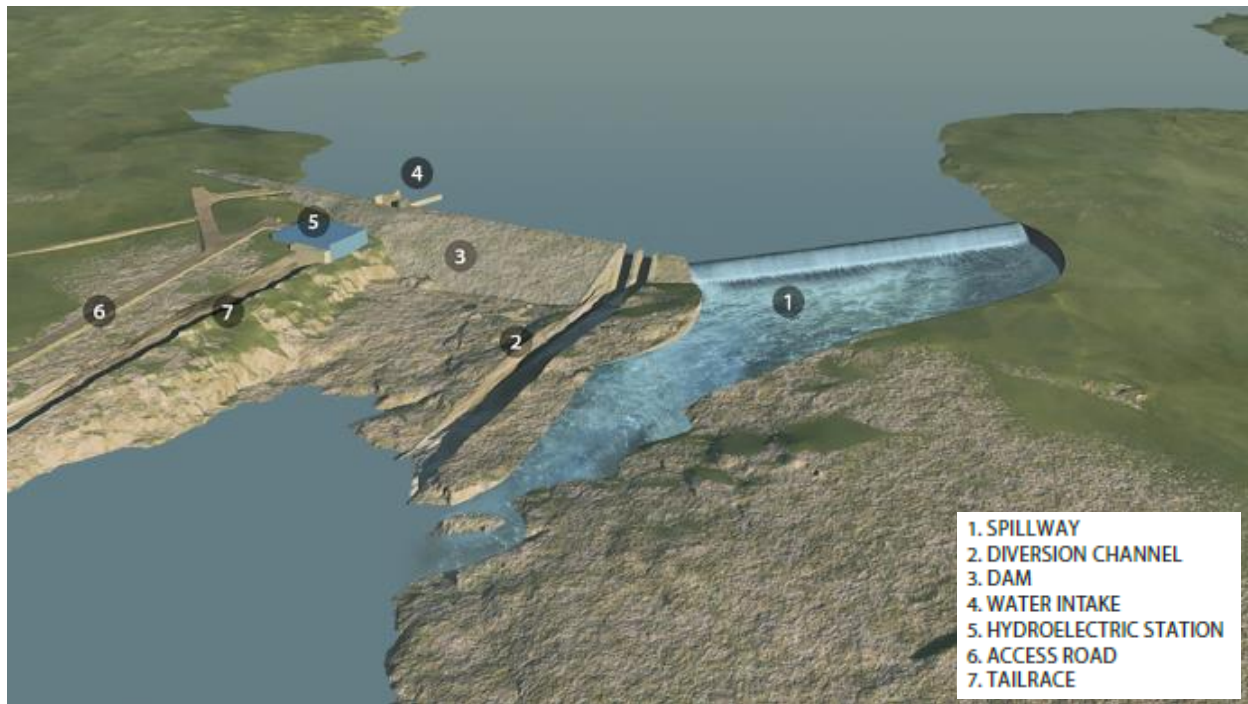
FIGURE 1: ILLUSTRATION OF THE INNAVIK HYDROELECTRIC PROJECT
