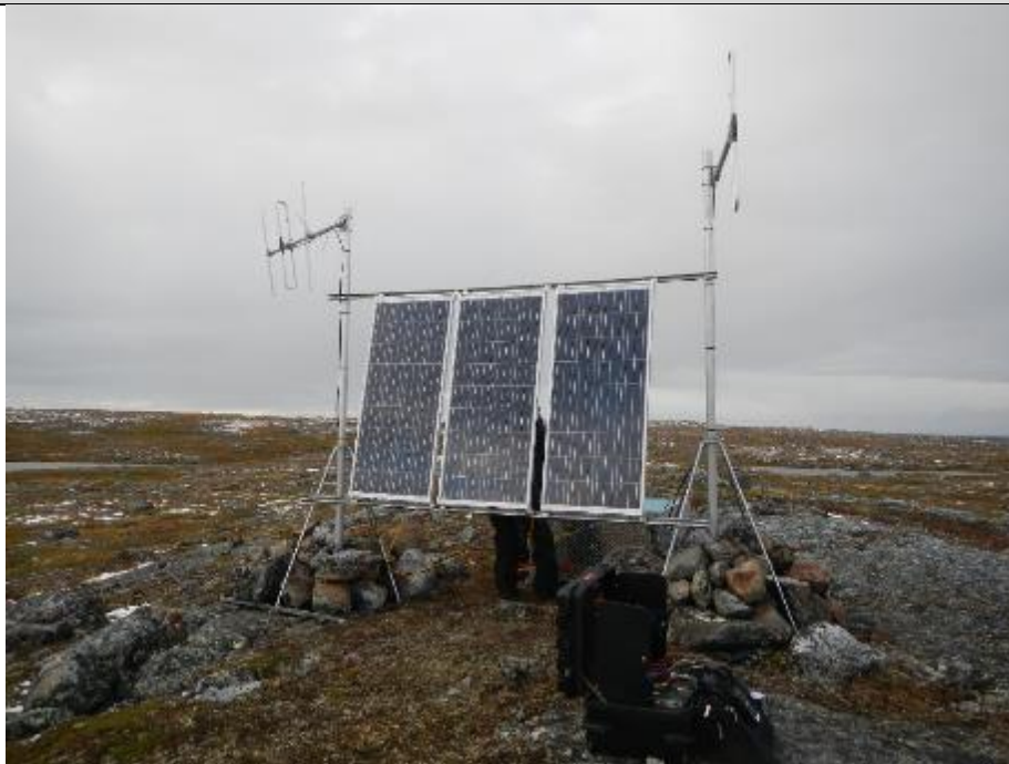
Figure 4. Photo of the repeater installed in 2013. The solar panels did not withstand the winter winds, so another model will have to be considered; photo: KRG.
