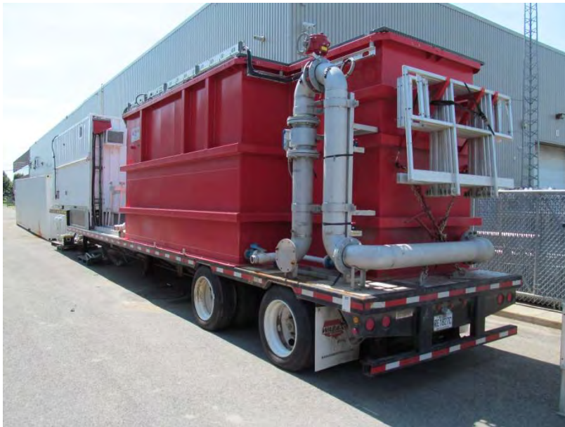
Figure 2 View of the Actiflo® Turbo Mobile Unit (Trailer Configuration)
