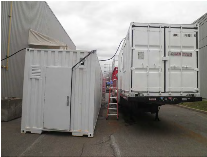
Figure 1 View of the Actiflo® Turbo Mobile Unit (Trailer Configuration)
