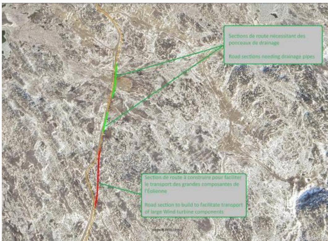
Section 2: The road sections where drainage ditches will have to be installed are indicated in green, while the road area to be modified (Access upgrade 2) to give it a straighter profile is shown in red.
