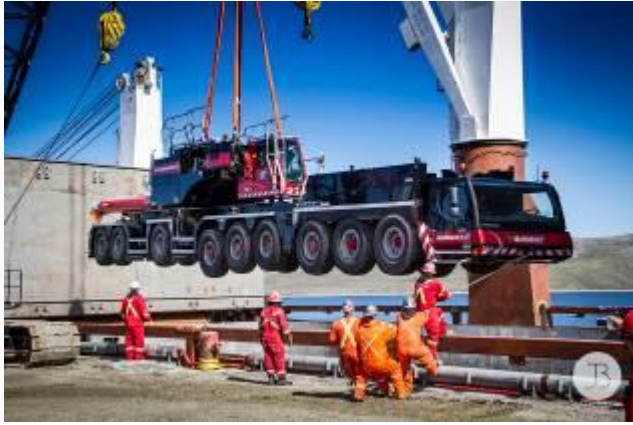
Unloading an 800-tonne crane from a ship in Nunavik
