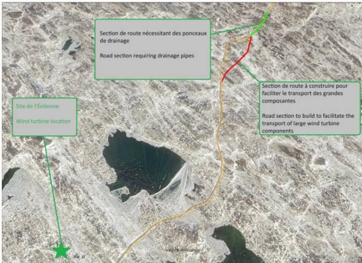
Section 3: The road sections where drainage pipes will have to be installed are indicated in green, while the road area to be modified (Access upgrade 2) to give it a straighter profile is shown in red. The green star indicates the planned location of the 3 MW wind turbine.
