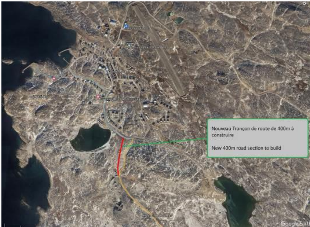
Section 1: The new 400m section of road (Access upgrade 1) is shown in red, and the existing section of road running along the rocky hill is shown in orange.
